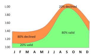
The relative distribution between valid and declined claims in a normal year. In the winter, the great proportion are associated with leaking drains etc., and in the summer, around 70% of valid claims are related to root induced clay shrinkage.
